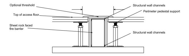
Note: For plenum spaces apply a bead of caulk at slab and foundation joints.
