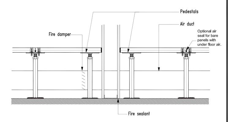
Note: For plenum spaces apply a bead of caulk at slab and foundation joints. Apply gasket material at floor interface and wall.
