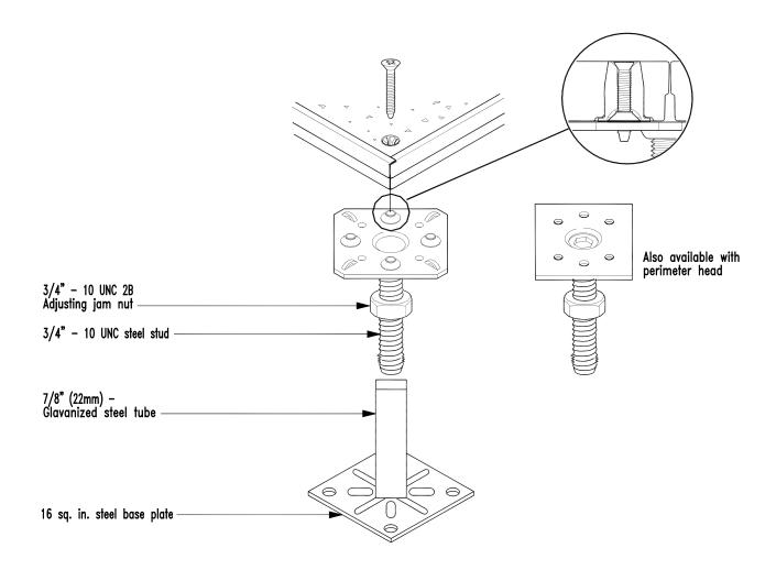
Note Standard pedestal bases are specified separately, for use with your choice of cornerlock field pedestal heads, or perimeter/transition pedestal heads.
