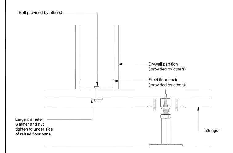
Alternative attachment method: If walls are secured at ceiling level, or stabilized by attached perpendicular walls, then powder actuated pins can be used to fasten floor track to the surface of the TecCrete panel in combination with construction adhesive. Final wall calculations and attachment method to be provided by others.
