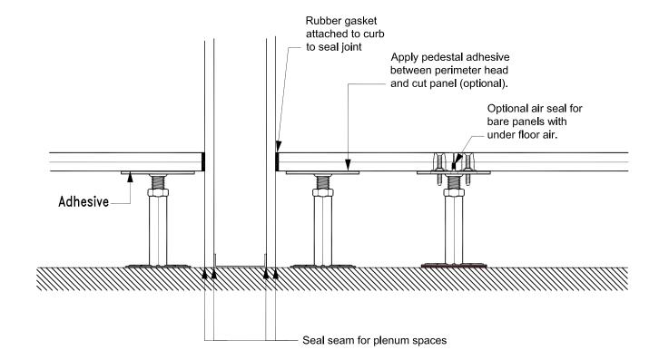
Note: For plenum spaces apply a bead of caulk at slab and foundation joints.
