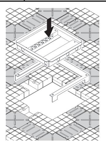
**NOTE:** Place electrical floor box along any seam on the Base Mat.
