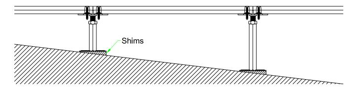
NOTE: Pedestals must be vertically level on all sides for a stronger and stable floor.
